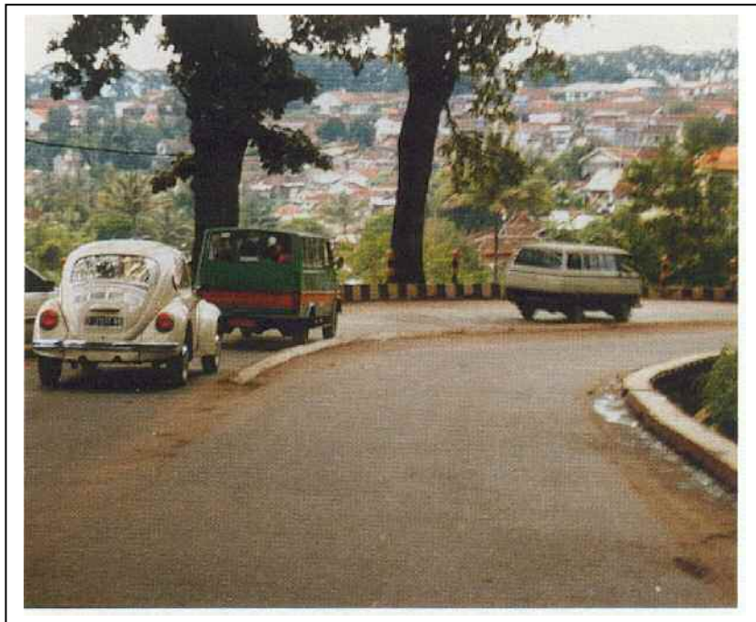
Figure 6-4: Example of self-enforcing measure: to reduce overtaking on bend
